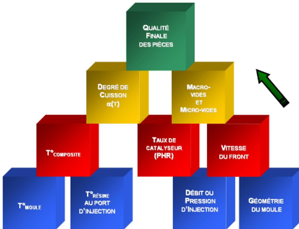
To control quality of produced parts, firstly "Machine Variables" and then "Process Variables" must be controlled well. Within the framework of Liquid Composite Moulding processes, these "Quality Criteria", "Machine Variables" and "Process Variables" are presented hereof.
